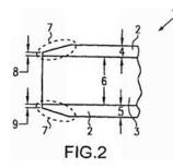
As can be seen from Figures 9 and 10, the space produced by tapers 7 is filled when two sandwich components 1 are joined. Material 15 is used, which is identical to the material of support elements 2. The protective covering 19 is produced by joining several sandwich components 1 together.
