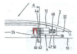
All that was claimed, however, was the adapter with the blind bore. No such bore is found in the accused product, where instead the bore passed through the adapter, which accordingly had no continuous bottom at the end of the bore.
